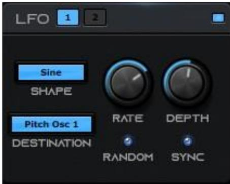
**The LFO (Low Frequency Oscillator) is used to create modulation of the sound.**
