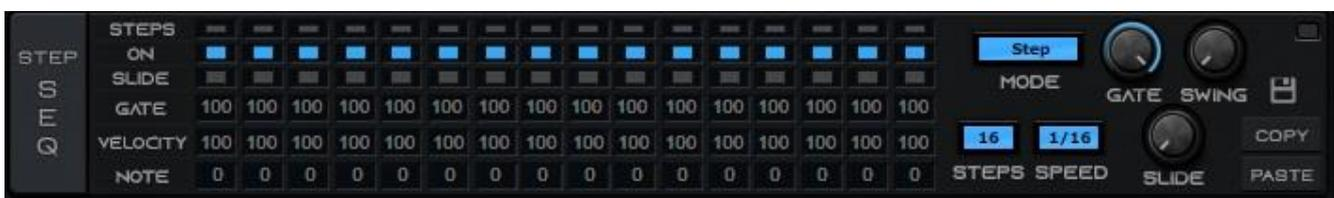
**STEPS:** Shows the currently played step when the Step Sequencer is enabled and you press a key.
