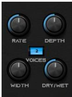
**RATE:** Sets the frequency of the LFO modulating the delayed signal.
