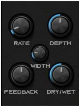
**RATE:** Sets the speed of the phaser (frequency)
