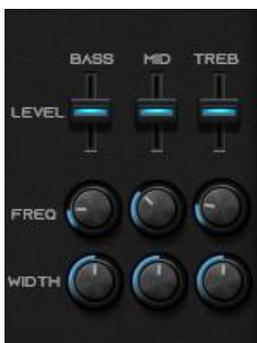
**LEVEL:** Controls the volume of each band (-18/+18 dB)
