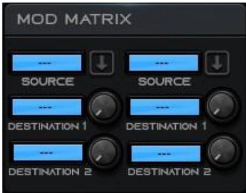
**The Modulation Matrix offers 2 assignable modulation sources with 2 destinations each and adjustable depth/amount.**
