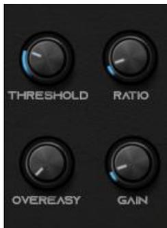
**THRESHOLD:** Determines at what dB level the compressor will begin working.
