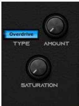
**TYPE:** Selects the distortion type between **Overdrive** and **HardClip**.
